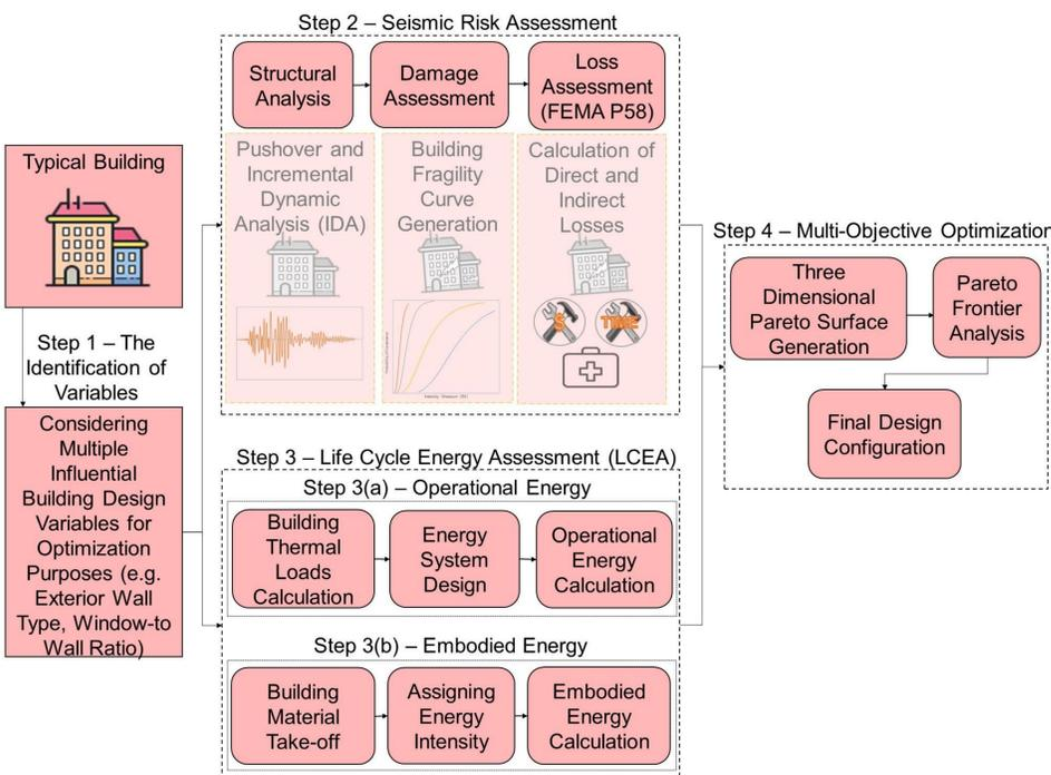
Figure 2. Schematic representation of the proposed multi-criteria decision-making framework
