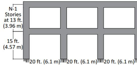
Figure 3. Schematic view of the simulated RC buildings
