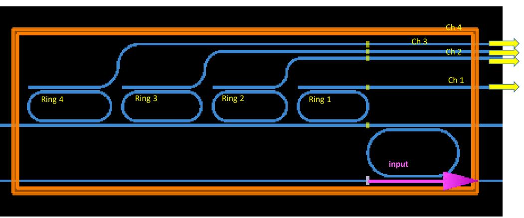
Wavelength (um) • The photonic chip comprised of cascade micro-resonators can create a multi-channel spectrometer with wavelengths precisely aligned with target molecular absorptions.
