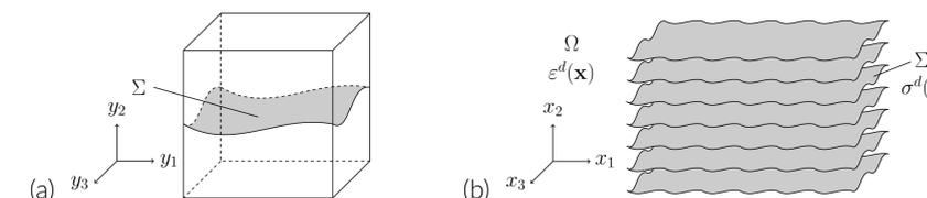
**Schematic of geometry:** (a) The unit cell,  $Y = [0, 1]^3$ , with microstructure  $\Sigma$ , a conducting sheet. (b) Computational domain  $\Omega$  with rescaled periodic layers  $\Sigma^d$  and spatially dependent surface conductivity  $\sigma^d(\mathbf{x})$ . The ambient medium has a heterogeneous permittivity,  $\epsilon^d(\mathbf{x})$ .
