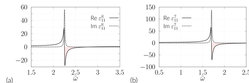
Plots of real and imaginary parts of matrix elements of  $\epsilon^{\text{eff}}$  as a function of frequency. (a)  $\epsilon_{11}^R$  for nanoribbons; and (b)  $\epsilon_{11}^T$  or  $\epsilon_{22}^T$  ( $\epsilon_{11}^T = \epsilon_{22}^T$ ) for nanotubes. The shaded area indicates the frequency regime for negative real part in each case.
