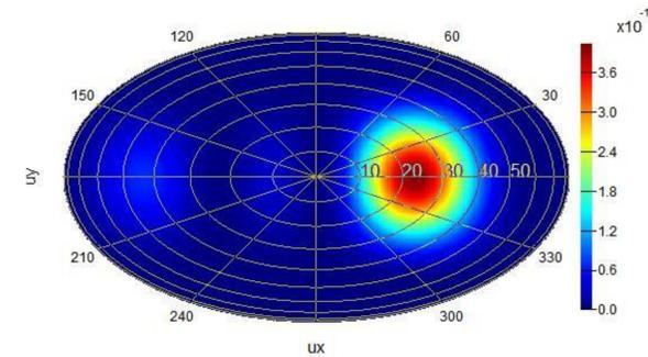
Far-field emission profile from the perovskite directional emitter (designed 23° emission)
