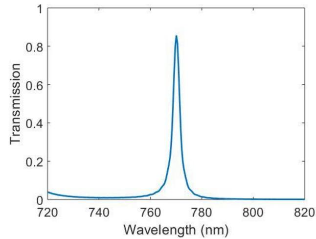
Transmission calculation of the cavity
